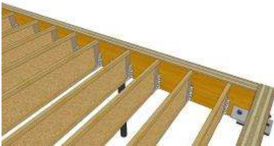
Floor Framing: I-joists (engineered wood)
